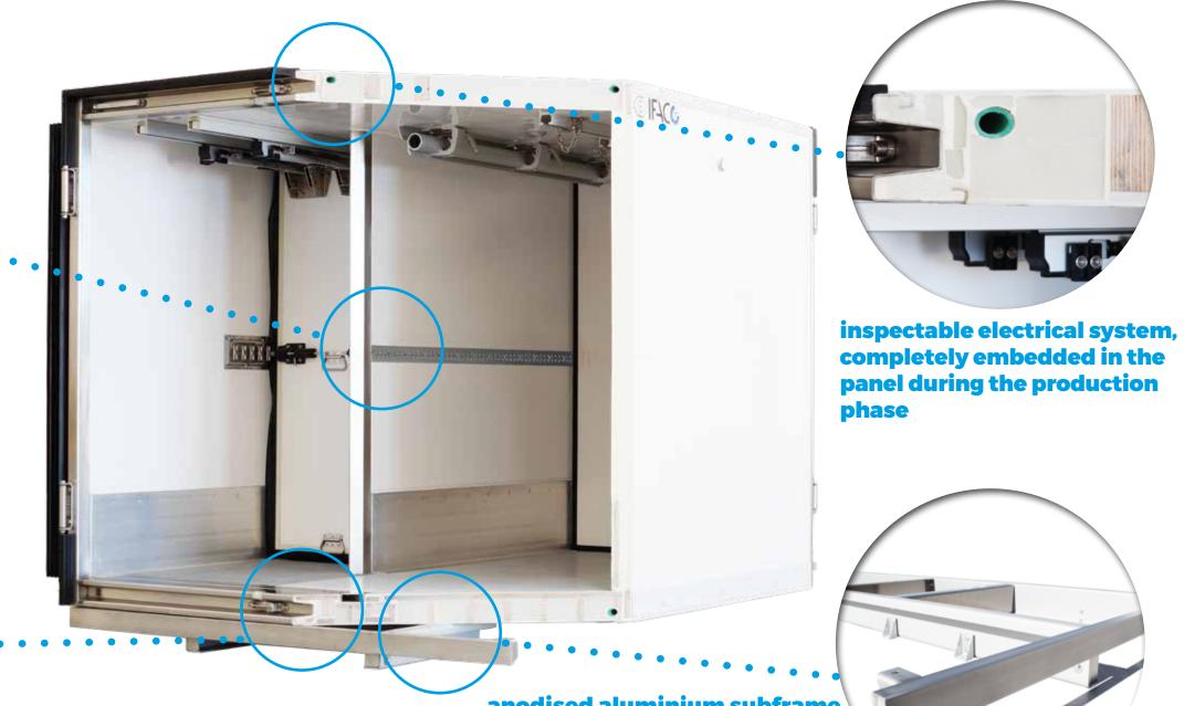
anodised aluminium subframe designed to reduce the weight of the vehicle and increase the maximum load
