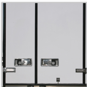
Inox rear locks and recessed/external handles and inox hinges
