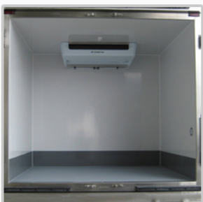
Inox rear frame built in the panels
